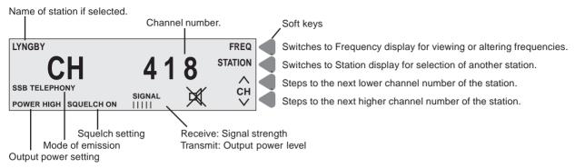
A channel number may also be keyed in directly from the keyboard. If the channel is not allocated to the station selected, the station name will disappear from the display.
