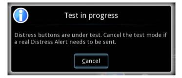
As long as the **Test in progress** window is showing, you can use Distress buttons connected to the system under test, without sending a real Distress alert.
