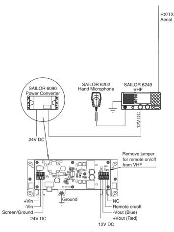
Figure 1: System configuration, example
