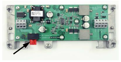
Figure 3: Replacing the fuse in the Power Converter
