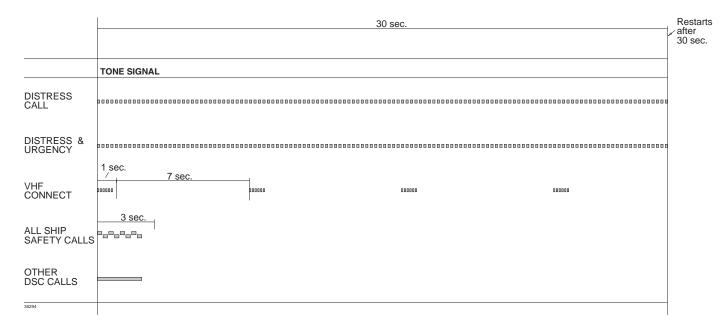
The tone signalling sequence is repeated every 30 seconds or until the DSC call is either read or answered. When handset is hooked off, there is a short tone every 30 seconds until call is read.
