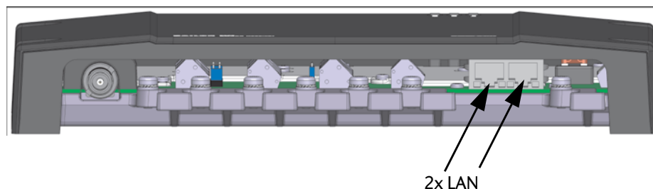
Figure 6-1: LAN connectors of the GNSS/DGNSS Receiver
