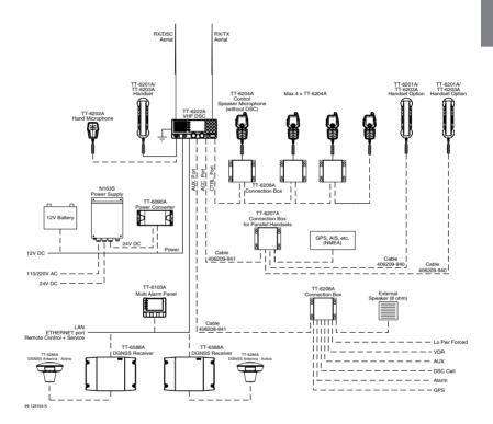
Figure 2: System configuration, example
