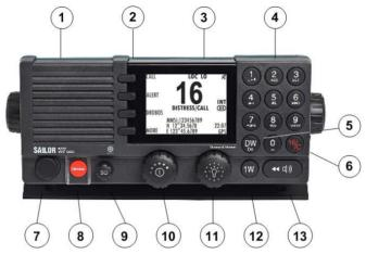
Figure 1: Controls on the front plate
