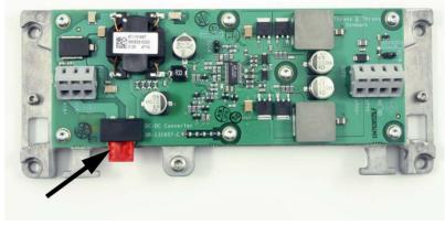
Figure 5: Replacing the fuse in the Power Converter
